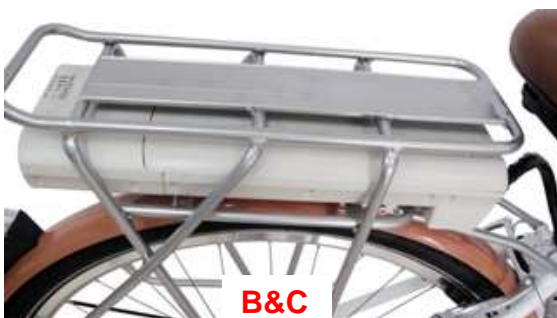
B&C. 36V / 9Ah Li Battery and Rack
