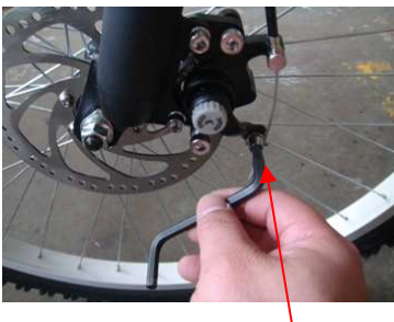
A: Loose the nut, release the brake cable B : Insert the cable into the brake lever
