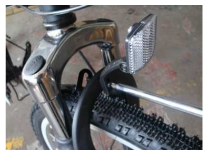
Install front reflector
