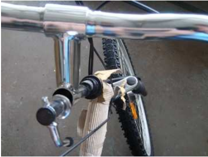
Insert the stem into head tube Secure the stem by quick release Adjust handlebar
