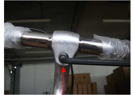
Insert the stem into head tube Secure the stem by quick release Adjust handlebar
