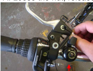
G Bell H: Rotate the lever I: Secure the brake lever
