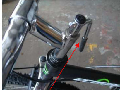
Insert the stem into head tube Secure the stem by quick release Adjust handlebar
