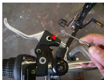
A: Loose the nut, release the brake cable B : Insert the cable into the brake lever
