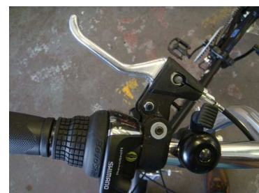
A: Loose the nut, release the brake cable B : Insert the cable into the brake lever
