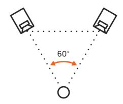
A two-channel stereo setup
