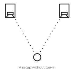
reflections from 100 Hz upwards. Using less toe-in will increase lateral reflections, usually resulting in livelier sound and a wider perceived sound stage. You can experiment with different toein angles to tweak the stereo image to your requirements or taste.
