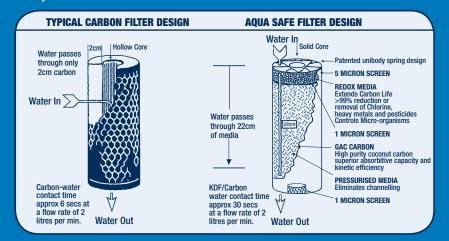
The **AS100 Bench top** filter mechanically filters out harmful cysts such as Giardia and Cryptosporidium while reducing or removing bacteria, chlorine and heavy metals. The carbon we use is produced from premium coconut shell ensuring a superior taste and quality than most standard carbon filters.
