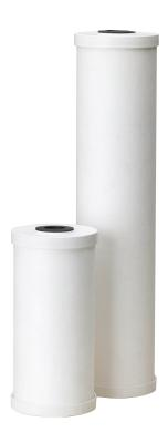
Pentair® Pentek® RFC Series Cartridges are constructed with a 70-micron porous polyethylene outer shell and durable polypropylene end caps. The 2-3/4" outer diameter cartridges have a polypropylene core and the 4-1/2" outer diameter cartridges incorporate a spun polypropylene core. Sandwiched between the outer shell and the core is a bed of granular activated carbon (GAC).
