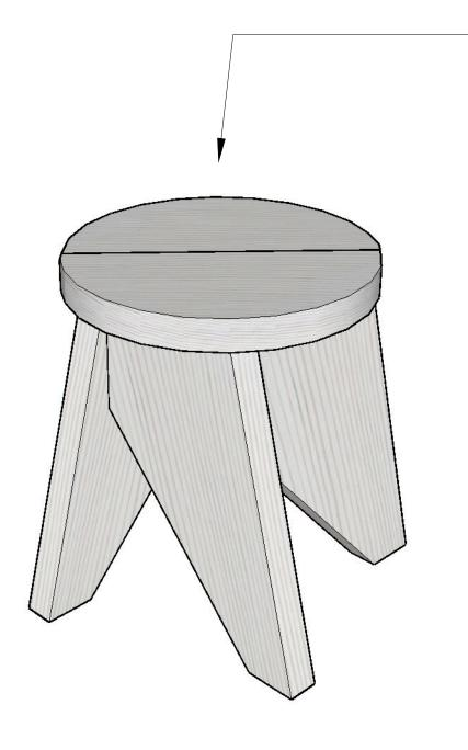
STOOL CAN BE LEFT RAW OR FINISHED WITH WAX, STAIN, PAINT OR POLYURETHANE.
