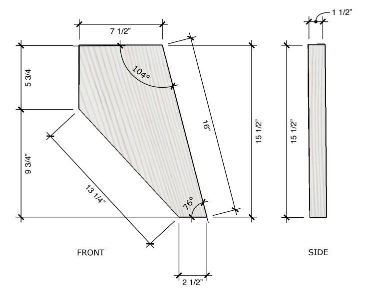
SEAT MADE OF 1.5" THICK 2x8 OR 2x10 MATERIAL (SPRUCE, PINE OR FIR RECOMMENDED)
