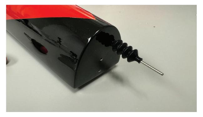
This photo shows the proper installation of the water rudder, pushrod, and seal. On the interior end of the pushrod, install the ball link.
