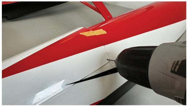
Then we remove the hatch, and apply a waterproofing bead of caulk or Gorilla CLEAR BOND glue as shown. Then install the hatch with screws.
