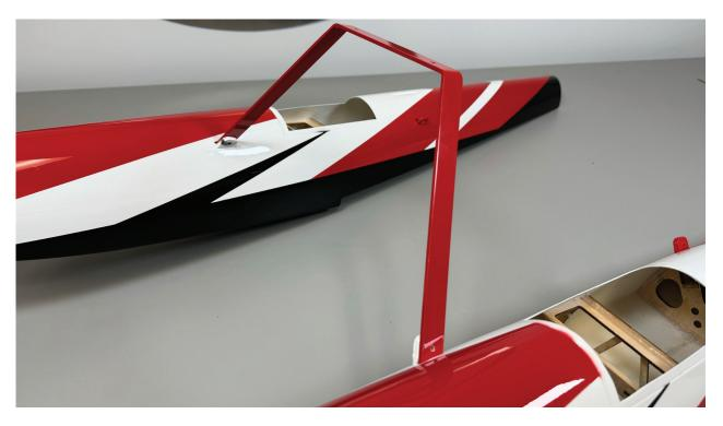
The struts asemble with 3MM bolts. Look carefully to find which struts have female threads for the bolts to screw into. Use a drop of blue Loctite thread locker on each of these bolts. NOTE: Now is a conveneient time to run your servo extension wire into the float, if you use the nearest slot which the strut inserts into, you can insert the servo plug through the slot and only make a small clearance of the slot to accommodate the servo wire.
