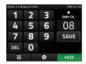
The Mystic 2 is equipped with DMX operation and utilizes three channels. To assign the DMX Channel, open the menu and select "DMX ADDRESS". Using the keypad, enter your desired DMX channel and press save. Your DMX channel is always visible in the top right corner of the screen.
