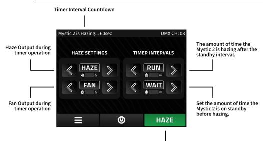
To access the timer settings, open the menu and select "SET TIMER". Using the diagram to the left, set your desired parameters and press haze to begin. To cancel the timer operation press conce.
