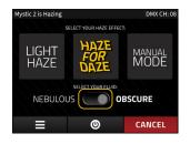
Your Mystic 2 is equipped with the unique ability to switch between 2 fluids to achieve a variety of effects. Prior to hazing it is important to "select your fluid" to ensure the heater is vaporizing your haze at the optimal temperature. Simply use the switch on the haze screen to designate your fluid.
