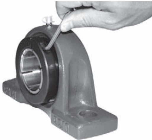
Fig 14.11 Installation of NU-LOC units
