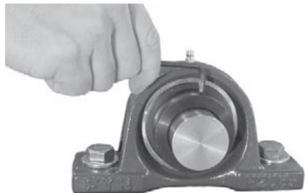
Fig. 14.10 Installing eccentric locking collar
