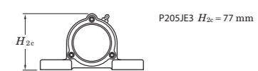
Forms and dimensions of H 2c of P205JE3 (housing with cast iron cover) are shown below.
