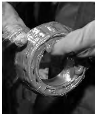
Fig. 23. Grease can easily be packed by hand.
