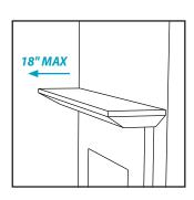
MantelMount can be installed in standard drywall using studs or to brick/stone using concrete anchors.
