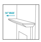
MantelMount can be installes in standard drywall using studs or to brick/stone using concrete anchors.
