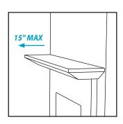
MantelMount can be installed in standard drywall using studs or to brick/stone using concrete anchors.
