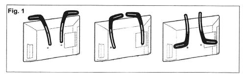
See Fig. 1 for examples of multiple configurations you can use to adapt the Soundbar Brackets to match your soundbar mounting holes. Use the configuration that works best with your soundbar.
