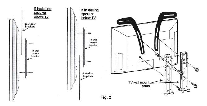
Insert the Soundbar Brackets in between the back of your flat panel and your wall mount, as shown in Fig. 2. You will be using your wall mount panel screws to affix the Soundbar Brackets to your TV. Secure with one bolt in each bracket as demonstrated in the diagram. Do not screw all the way as final adjustments may be necessary.
