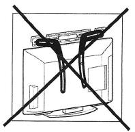
**CAUTION!:** PLEASE DO NOT MOUNT YOUR SOUNDBARS USING SOUNDBAR BRACKETS IF YOUR PANEL IS NOT WALL MOUNTED. MOUNTING TO A TV ON A PEDESTAL IS A TIPPING RISK. THIS COULD CAUSE DAMAGE TO EQUIPMENT AND POSSIBLY LEAD TO PERSONAL INJURY.
