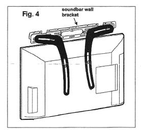
B) If your soundbar is already affixed to a soundbar wall bracket Using hardware from bolt bag, attach your soundbar's wall bracket to the Soundbar Brackets as shown in Fig. 4.
