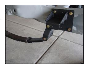
8. Install rear spring shackles (SAS001-6) into the rear shackle brackets using 9/16" x 4½" bolt and locknut. Install new front leaf springs (NOT SUPPLIED IN KIT) into front spring hanger and rear shackles using 9/16" x 4½" bolts, nuts without washers. Recommended springs: 73-87 Chevy Front springs with 88-91 bushing and sleeve kit.
