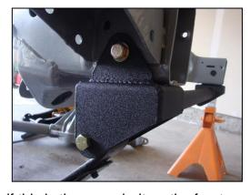
will not align with the front crossmember; if this is the case, bolt on the front cross-member using the side ear tabs, and then mark and drill new ½" holes.
