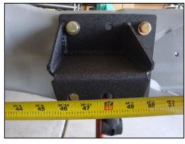
6. Repeat step 5 for the drivers side rear shackle bracket (SAS001-3). The long slot on the bracket should align with the manual transmission shift linkage.
