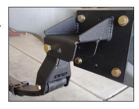
9. Strip the front axle housing of all factory shock and sway bar mounts. On Ford Dana axles, you will need to grind a notch in the casting for the drivers side inner U-bolt to sit in. Half the depth of the U-bolt will be adequate.
