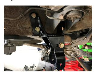
13. Install 18x130mm Bolts (1-1/16 Socket) followed by the 5/8x5.5" Bolts (15/16 Socket) through the front hanger and shackle to hang your leaf springs. 18mm Spring eye w/ Military Wrap goes Forward!!!
