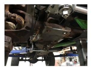
6. Install new front hanger, lining up the 5/8 bolt holes in front hanger and frame. Install frame spacer into frame opening and insert 5/8x4.5" bolt through holes in frame and install nuts.
