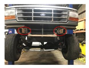
3. Check for cracks in common locations near the shackle hanger behind bumper.
