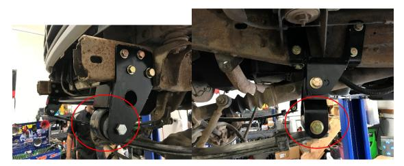
14. Install new U-bolts (7/8 Socket) and snug up to the axle, but do not make over tight. You will most likely have to trim the U-bolt plate on the driver's side to clear the differential.
