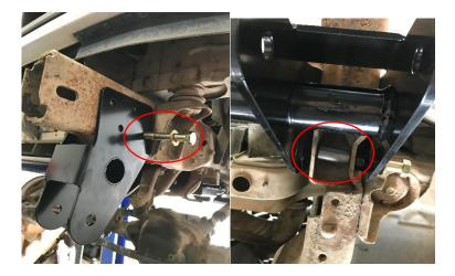
7. Measure 55.5" from center eye of factory rear spring hanger to center of new front spring bolt hole to set where the front hanger should sit.
