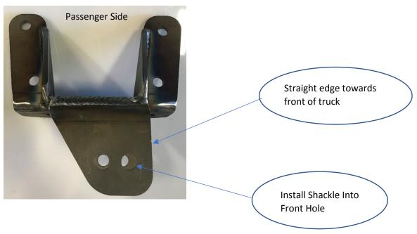
10. To install the shackle hanger you will need to remove the factory rivets; there are many ways to remove the rivets.
