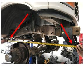
8. Center punch and drill 1/2" holes (on both sides of frame) in new front cross member locations as marked by the 1/2" holes in the front cross member (drilling a pilot hole and using oil and a sharp step bit will save you a massive amount of time). Install 1/2x1.5" bolts ,nuts ,and flat washers to hanger through frame. Be sure to use red Loctite and torque to specifications.
