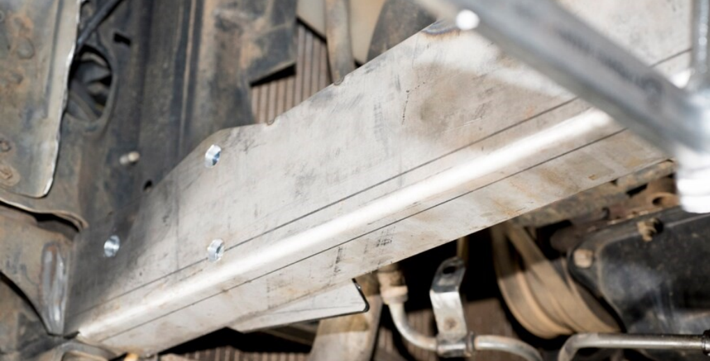
Check Frame plate lines up with frame tubes
