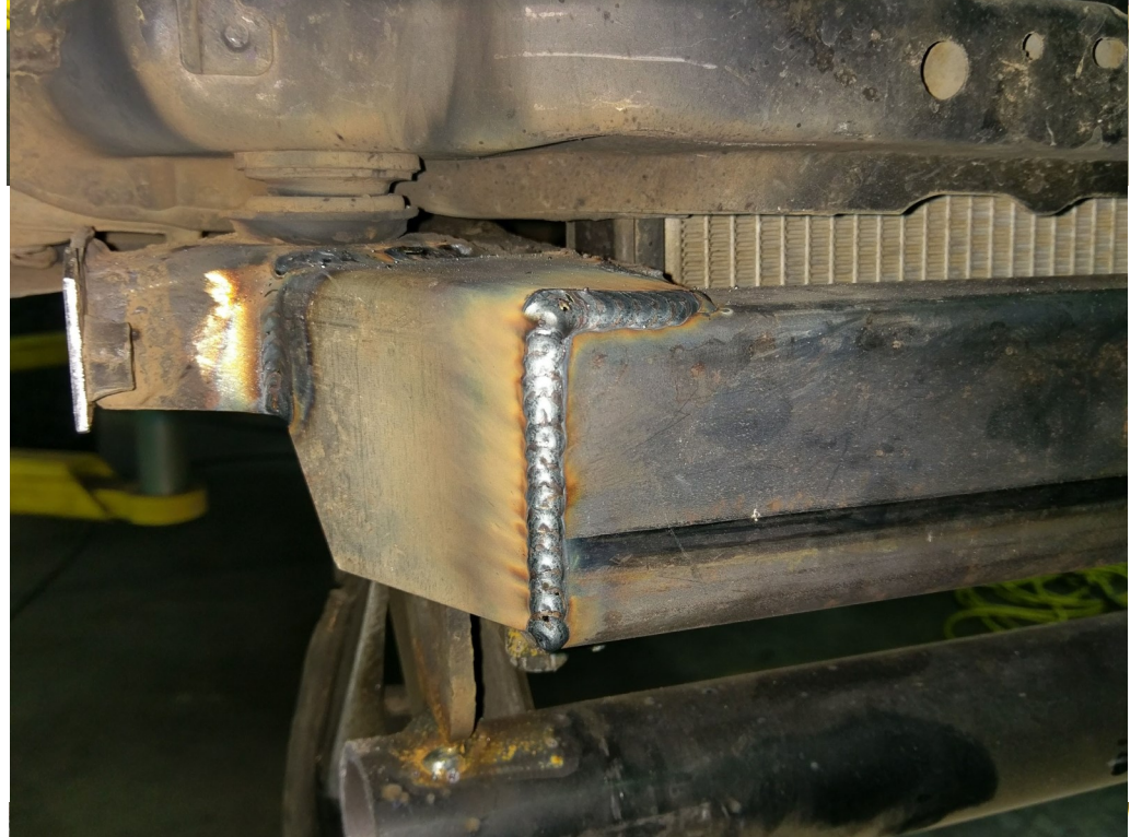
Weld in front frame rail reinforcement
