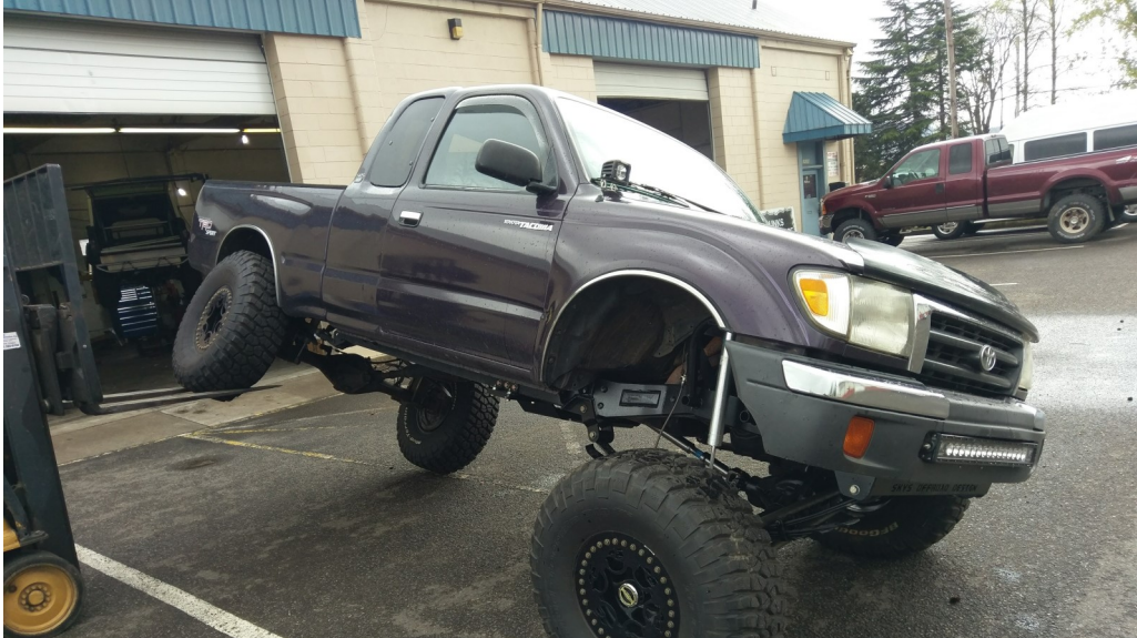
Flex test to measure for shocks and check for clearance issues.
