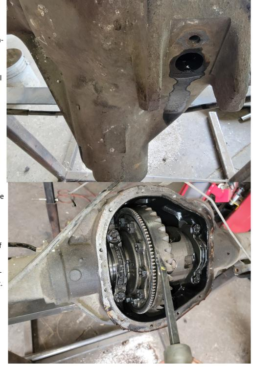
Next remove the axle shafts, diff cover and differential carrier from your 10.5 axle..
