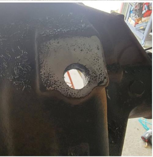
Thoroughly clean any debris from the inside of the axle.
