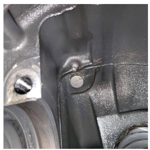
Install the sensor and check the distance between the sensor and the tone wheel.
