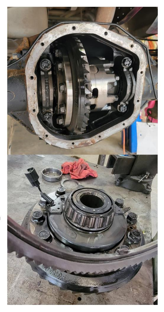
Press the tone wheel on by lightly tapping it on with a rubber or brass hammer, working your way around to work it on evenly.
