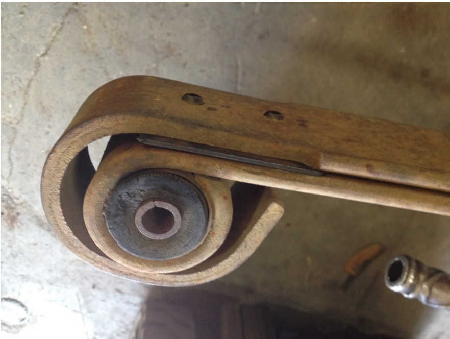
Military wrap side of the leaf spring with isolator installed.
