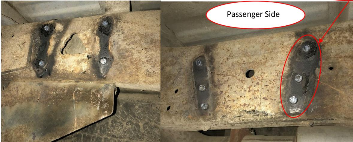
3. Install Rear Shackle Flip (there is a left and right, line holes in frame up with bracket so it runs close to parallel with the frame) secure using 1/2-1.25" bolts. Bolt Conversion Boomerang shackle with bushings and sleeves in forward holes using 9/16 Bolts.
