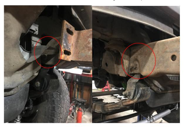
4. Remove Rear Leaf Spring Hanger Bolts (3/4 Socket) and Front Shackle (15/16 Socket)
