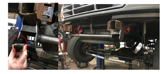
7. Measure 55.5" from center eye of factory rear spring hanger to center of new front spring bolt hole to set where the front hanger should sit. \*Note this is for a 56" long stock spring, if you have an aftermarket spring that measures shorter you will need to adjust to compensate for that.
