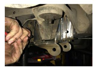
12. Install shackle bushings and sleeves, grease liberally. After pins are installed, use 9/16x5.5" bolts to hang the
