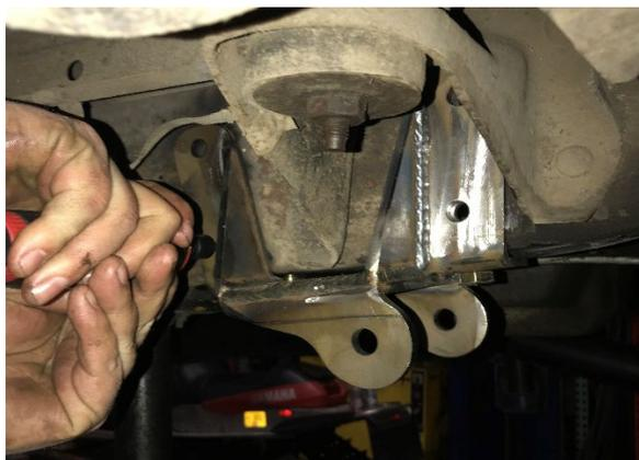
12. Install shackle bushings and sleeves, grease liberally. After pins are installed, use 9/16x5.5" bolts to
