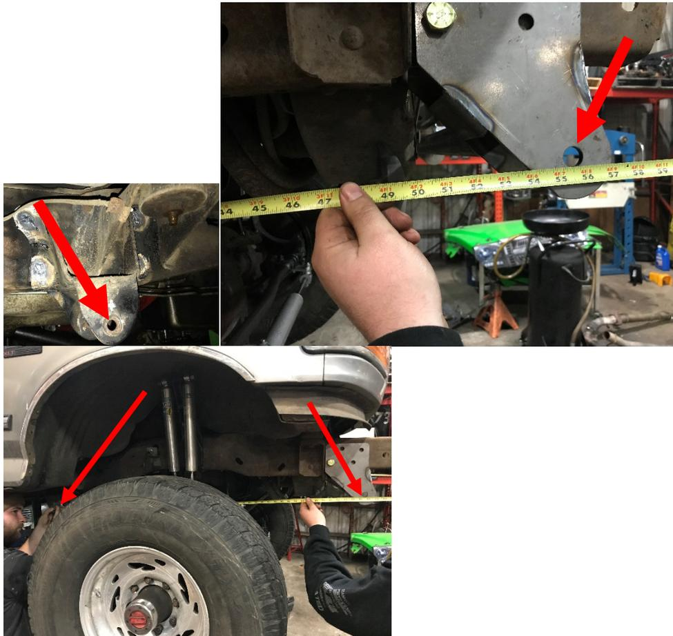
8. Center punch and drill 1/2" holes (on both sides of frame) in new front cross member locations as marked by the 1/2" holes in the front cross member (drilling a pilot hole and using oil and a step bit will save you a massive amount of time). Install 1/2x1.5" bolts ,nuts ,and flat washers to hanger through frame. Be sure to use red Loctite and torque to target specifications.
