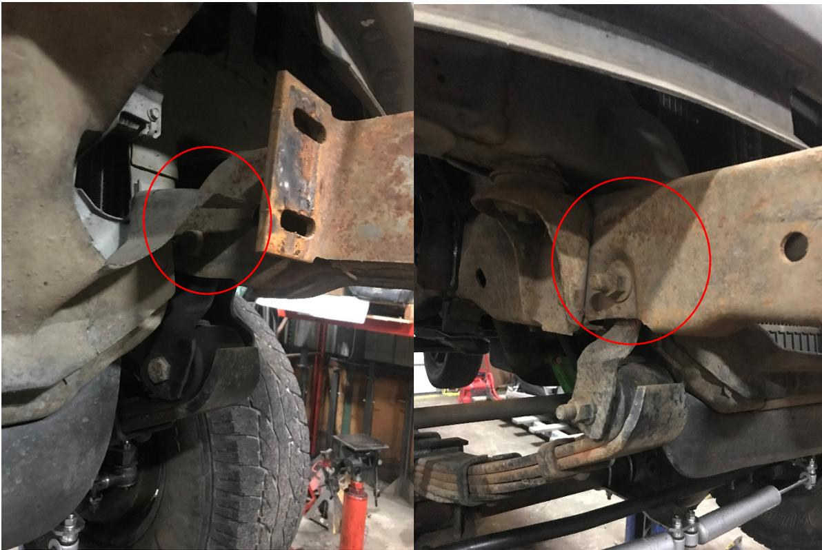
4. Remove Rear Leaf Spring Hanger Bolts (3/4 Socket) and Front Shackle (15/16 Socket)
