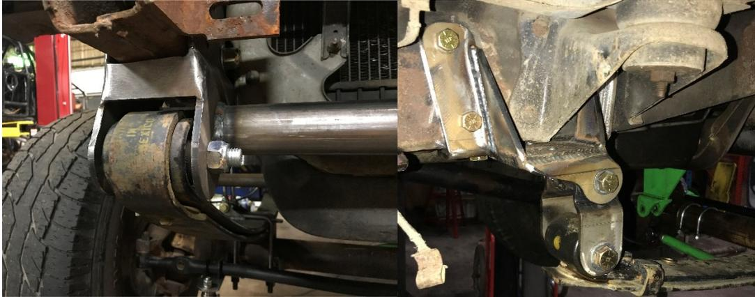
14. Install new U-bolts (7/8 Socket) and snug up to the axle, but do not make over tight.
