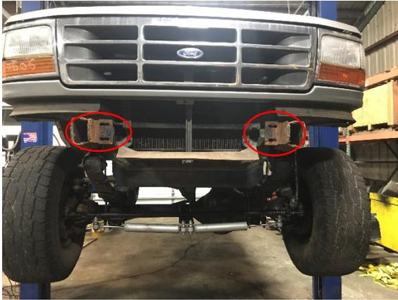
3. Check for cracks in common locations near the shackle hanger behind bumper.
