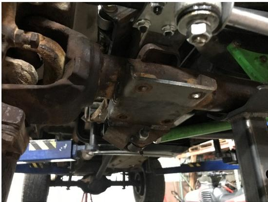
6. Install new front hanger, lining up the 5/8 bolt holes in front hanger and frame. Install frame spacer into frame opening and insert 5/8x4.5" bolt through holes in frame and tighten bolts snug, you will torque all hardware at the end of installation.
