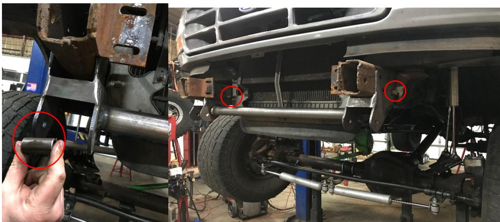
7. Measure 55.5" from center eye of factory rear spring hanger to center of new front spring bolt hole to set where the front hanger should sit.
