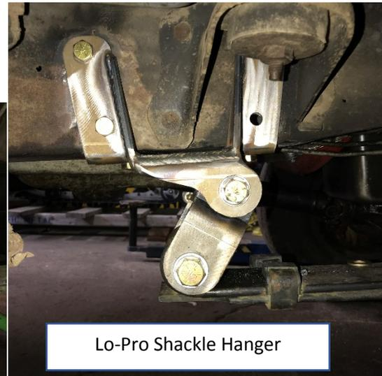
10. To install the Lo-Pro shackle hanger you will need to remove the factory rivets; there are many ways to remove the rivets. We recommend scarfing them off with a torch and using an air hammer to punch them out of the frame.
