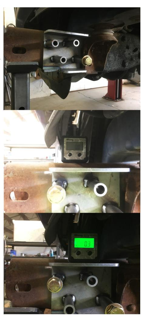
With the box kit properly aligned to the frame use a 1/2" transfer punch to locate the remaining holes.
