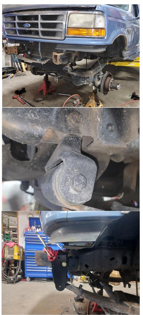
9. To locate front hanger after installing 5/8" pilot bolts, Measure 51.5" from center of rear spring bolt to center of new front spring bolt hole, clamp front hanger in place so it doesn't move. If using shorter than 52" factory length springs this dimension will need to be changed in order to fit correctly.
