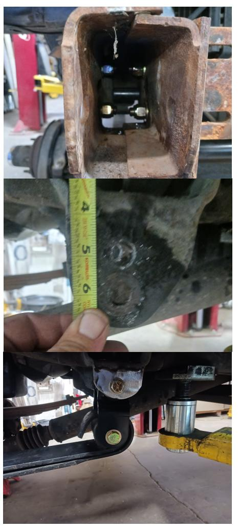
13. Check to make sure brake lines are not stretched. You may have to bend the hard line at the calipers toward the frame and/or bend down the tab that holds lines at frame.
