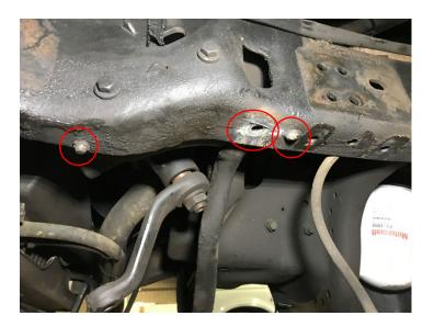
5. Install  $\frac{1}{2}$ -20-1.5" bolt for panhard bracket, tighten on the frame, clamp bracket to cradle and mark the three holes on the cradle to drill.
