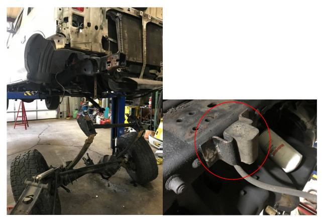
4. Swap out pitman arm to accept the drag link end. Remove line-up pegs and rivet on drivers side to prep for panhard bracket installation.
