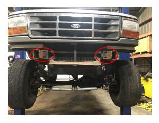
3. Remove everything on your front end. Pitman arm, springs, spring hangers, swaybar mounts, upper shock mounts, shackles, driveline, and bumpstop brackets.
