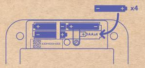
Insert 4 x AA new alkaline batteries matching the + - symbols as shown.
