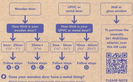
Metal linings may interfere with the microchip reader. Test whether your door has a metal panel by drilling a small hole in the middle of the intended cat flap location. If your door contains metal, follow the retuning instructions at the end of installation. If your door contains metal, ensure that you remove the batteries before starting installation. PLEASE NOTE Fitting instructions for glass and walls are not covered in this manual
