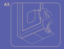
We recommend the bottom of the cut out template is approximately level with your pet's stomach.
