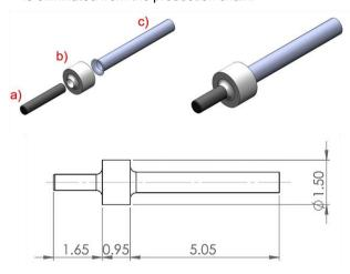
Fig. 1. Micro assembly three dimensional model and main dimensions in mm. (a): Magnet rod. (b): TPE micro-ring. (c): Aluminum cantilever.
