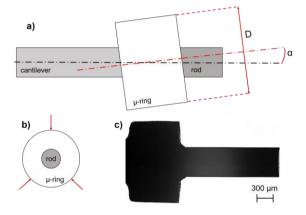
Fig. 3. (a): Measurement scheme. The diameter D and the angle  $\alpha$  are indicated. (b) The three circumferential measuring positions. (c) Micro assembly as viewed by the optical CMM.
