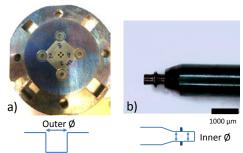
FIGURE 4: a) Mold plate containing 4 cavities; b) pin entering the cavity during injection molding production of the suspension ring. **DISCUSSION AND RESULTS**
