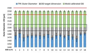
FIGURE 8: Quality conformance assessment of TPE micro rings. Error bars on TPE OD indicate experimental measuring uncertainty. Error bars on the calibrated OD mold cavities dimension indicate expanded uncertainty U=2,9 µm.
