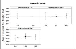
FIGURE 5: Main effect plot of measured suspension rings Outer Diameters.
