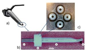
FIGURE 1: a) high performance DJ cartridge, b) (b-1) magnet (b-2) TPE suspension ring (b-3) Aluminum cantilever (b-4) Diamond tip; c) 2D visual inspection of produced suspension rings.
