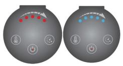
2.2 Constant temperature mode: adjustable temperature range 45 °C -65 °C, default temperature 65 °C, the 1st red light is 45 °C, each red light lit later increases by 5 °C. As shown in following picture
