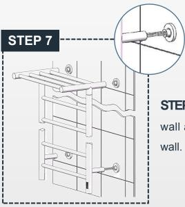
**STEP7:** Connect the core wire from the leg to the power wire inside the wall and then lie the towel rail against the mounting seats fixed on the wall.
