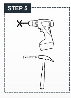
**STEP 5:** Make the holes with an electric driller; Be sure to drill a hole for the core cable going from the mounting feet to the wall. And use a hammer to knock plastic wall anchors into wall completely.
