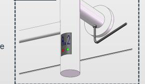
**STEP 8:** Use the Allen wrench to install the hex screws into the holes of all the tubes to complete the installation.
