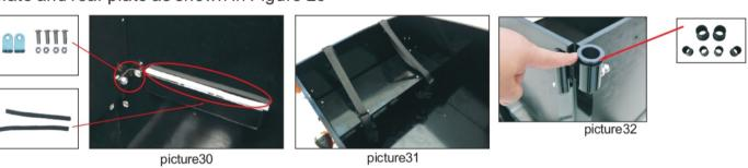
Seat plate assemble on box front side, fixed on the side panel on both sides, box front seat plate put article shockproof both front side < as shown in figure 30,31>;
