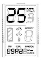
**Note**: The motor output power continues to decay when the wheel speed reaches or exceeds the set value. For cycling safety, it is recommended to set the speed limit at 25Km/H or below.
