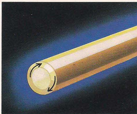
Fig. 1. Solid pole pin with circulating eddy current.
