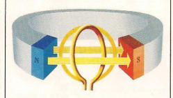
In neutral, the coil is by-passed by the magnetic field and no signal is generated. But when the stylus and cantilever shift into the second position, the coil contacts the magnetic field and a signal is induced.
