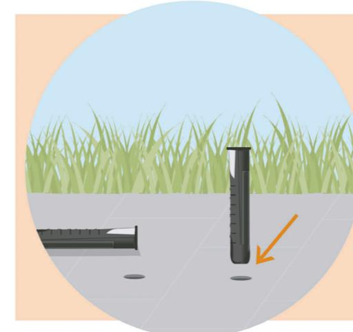
**EN:** Attention: For stone/concrete/tiles etc., place the plugs in the drilled holes. **Do not use a plug if you have a wooden base.**
