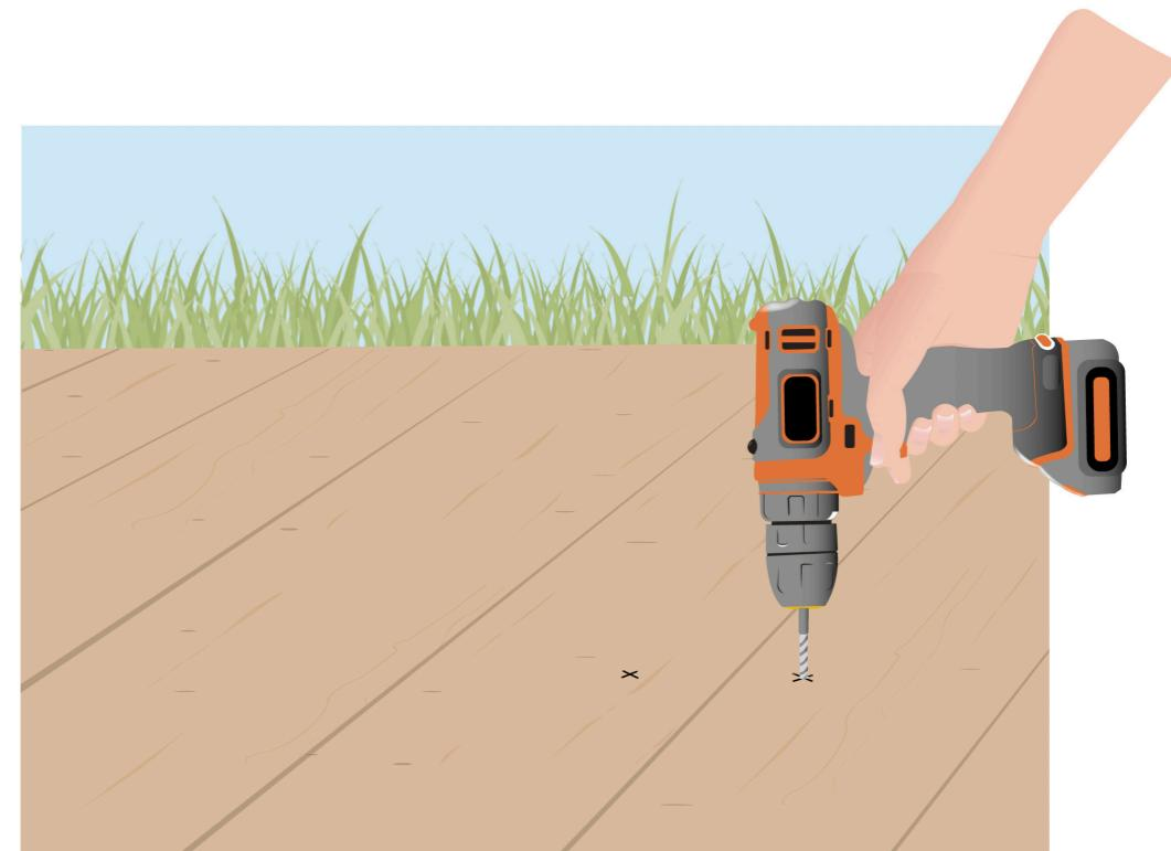
**EN:** Now mark the two points where holes are to be drilled in the substrate. Drill these holes with drill size 10/ fractional size 19/64 (for stone/concrete/tiles) or drill size 4/ fractional size 1/16 (for wood). Drill the holes approximately 6 cm/ 2.36 in. deep.
