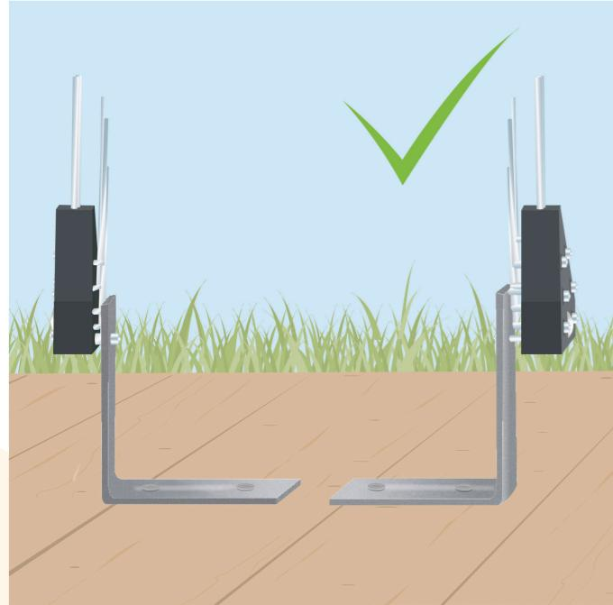
**EN:** Now screw the corner brackets to the ground. Then unscrew the hinge blocks from the standard hinge anchors and attach them to the corner brackets as illustrated.
