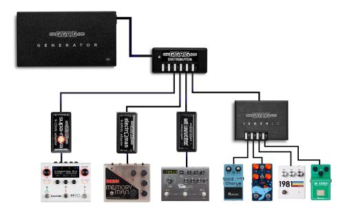
The ISOx4 LC outputs are based around our award-winning Virtual Battery technology. Each output uses a tiny toroidal transformer where the positive and the negative are both isolated and delivers exactly what the pedal needs to operate at their best.
