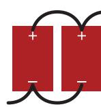
System Voltage: 48V System Capacity: 60Ah
