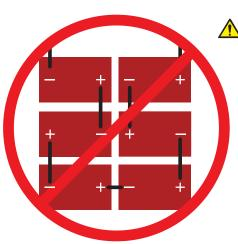
Do NOT install batteries in Series. This may permanently damage the battery.
