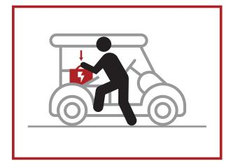
Place GC2 48V Lithium-Ion in golf vehicle battery compartment.
