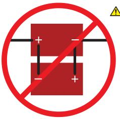
Do NOT install batteries in reverse polarity.
