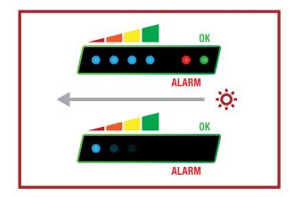
• Turning Off: Press and hold the Status Button. All LEDs will turn on, then successively turn off from right to left. Once all LEDs are off, wait another 1-2 seconds, then release the Status Button.
