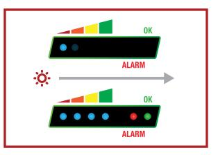
• Turning On: Press and hold the Status Button. LEDs will successively turn on from left to right. Once all LEDs are on, wait another 1-2 seconds and release the Status Button.
