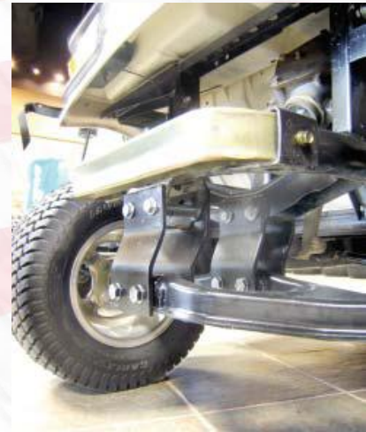
FRONT A-ARM RISERS notched on the rear
