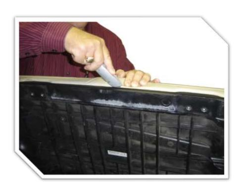
Carefully slit existing vinyl upholstery away from plastic base using a sharp utility knife. Do this around the entire perimeter of the seat.
