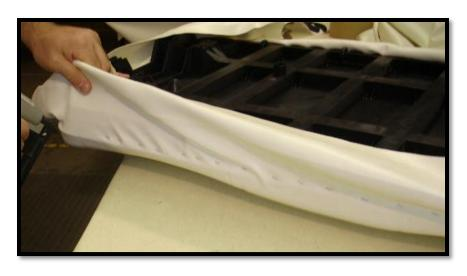
On clean work surface, turn over cushion and staple through vinyl into plastic base. Hint: staple long sides first, starting in the center and working out to both ends.
