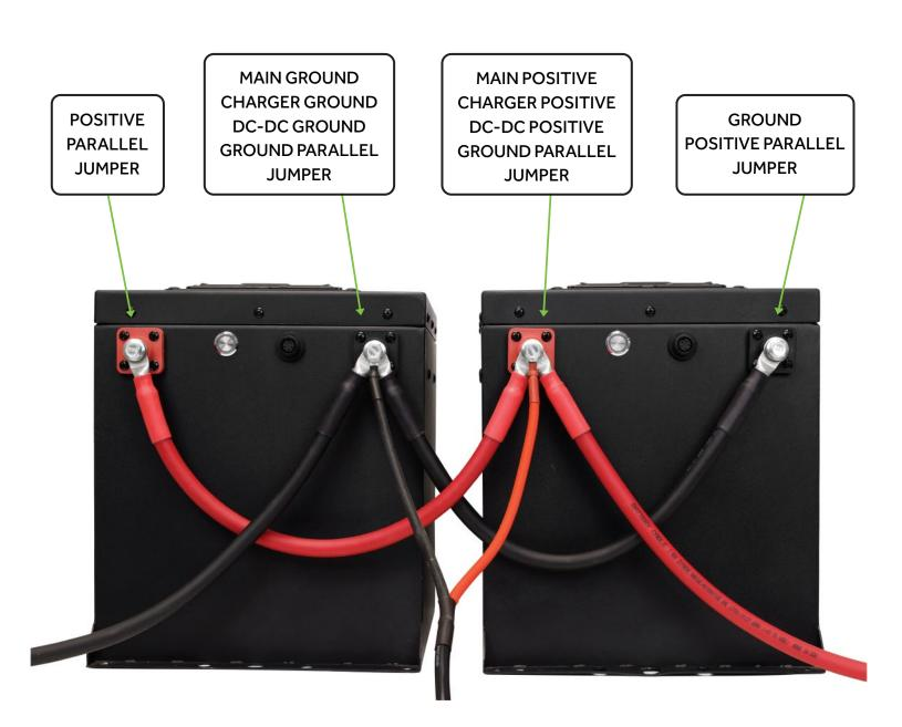
\*THE MAIN POSITIVE AND MAIN NEGATIVE SHOULD BE CONNECTED ON OPPOSING BATTERIES, AS SHOWN.
