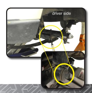
Reinstall factory leaf spring above the axle and install rear lift block under the leaf spring as shown. Check spring bushings for rust and wear. Replace if necessary.
