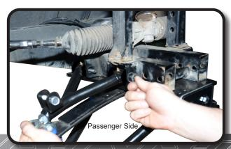
Using 3/8" allen wrench attach spindle to upper and lower A-arms. Repeat on other side.
