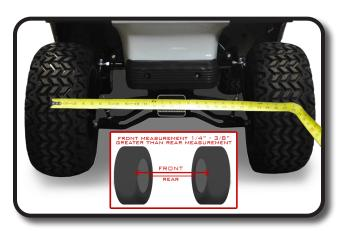
NOTE: After the first hour of drive time, re-check all lift kit components and alignment. Regrease the fittings, check the alignment and ensure all lift kit hardware is secured for safety after 50 hours of recurring use.
