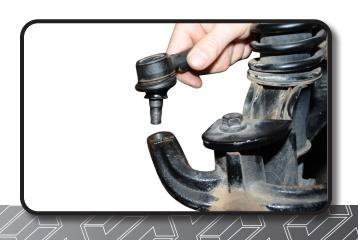
Using a 15mm socket and wrench remove hardware from top of the shock and from the lower control arm. Remove factory suspension assembly from cart. Retain hardware (factory suspension will not be reused).
