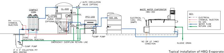
Typical installation of HBG Evaporator
