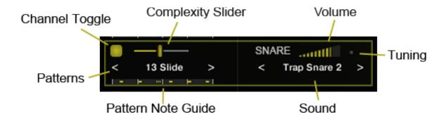
Only one channel can be selected at a time, and is indicated by a yellow rectangle outline. You can select a channel either by triggering its corresponding pad on the interface, or by clicking the channel name (for example, "SNARE").
