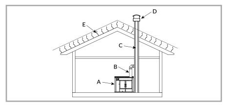
Picture 2 - Components of the chimney. A= Thermal cooker B= Conjunction or fume conduct C= Chimney hood D= Chimney pot E= Reflow zone
