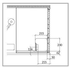
Picture 11 - Position of the rear hole for the passage of the air intake conduct. Dimensions in mm.
