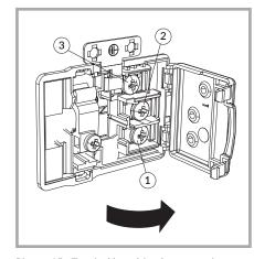
Picture 15 - Terminal board for the connection to the network: 1. Line 2. Neutral 3. Earth.
