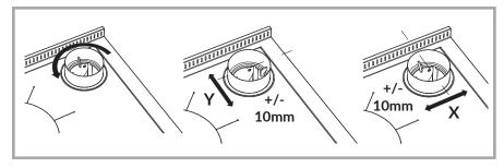
Picture 6 - Tolerance for flue outlet on the top and back. The tolerance depends on the orientation of the connector.
