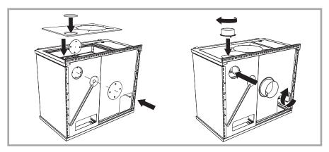
Picture 5 - Predisposition of the flue outlet (STP).
