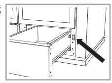
Picture 43 - Switch to light the oven.
