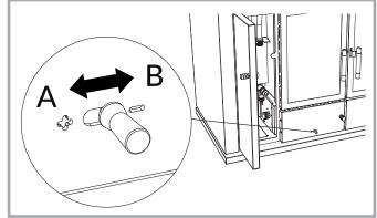
Picture 37 - Auxiliary regulation of the primary air: the valve is open at the position indicated with the letter A, while it is closed at the position indicated with the letter B.
