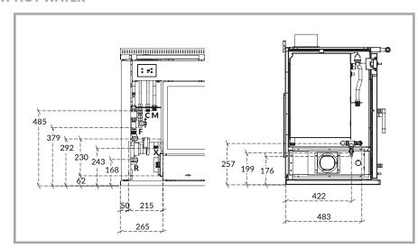
Picture 20 – Position of the connectors for the thermosanitary system. Position of the rear hole for the passage of the pipes.
