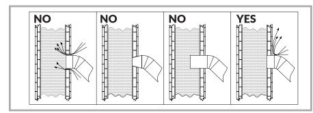
Picture 7 - Samples of correct and incorrect connection to the chimney hood.
