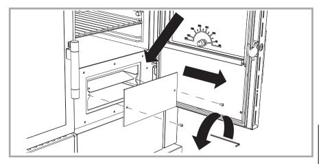
Picture 49 - Fume-circuit inspection.
