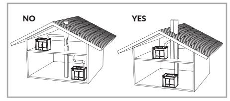
Picture 3 - Samples of correct and incorrect chimney connection.
