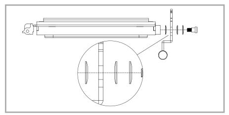
Picture 51 - Correct position of the rounded washers.
