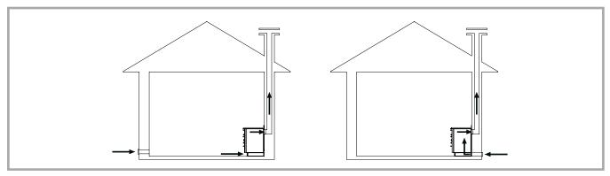
Picture 9 - Installation with air intake in the room and installation with external air intake connected directly to the thermal wood fired cooker.
