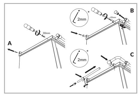
Picture 16 - Modification of the handrail.
