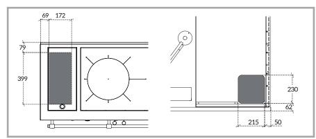
Picture 18 - Position of the lower hole for the passage of the pipes.
