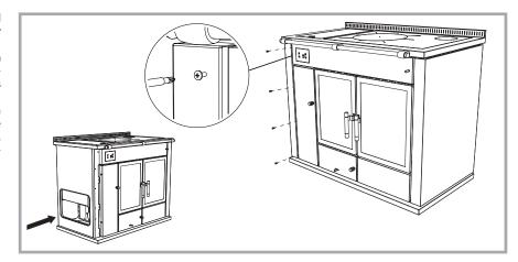
Picture 17 - Removing the boiler side with hole.
