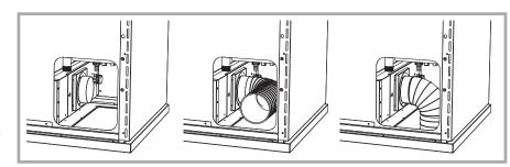
Picture 10 - Different connections of the air intake of the wood fired thermal cooker.
