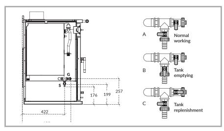
Picture 21 - Connectors for emptying and replenishment of the tank.
