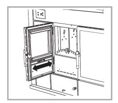
Picture 39 - Air adjustment for glass cleaning.
