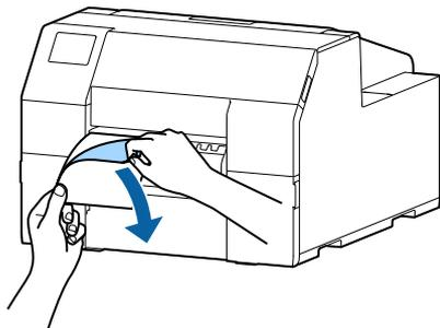
**14 Open the peeler cover.**
