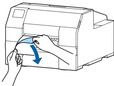
**12 Open the peeler cover.**
