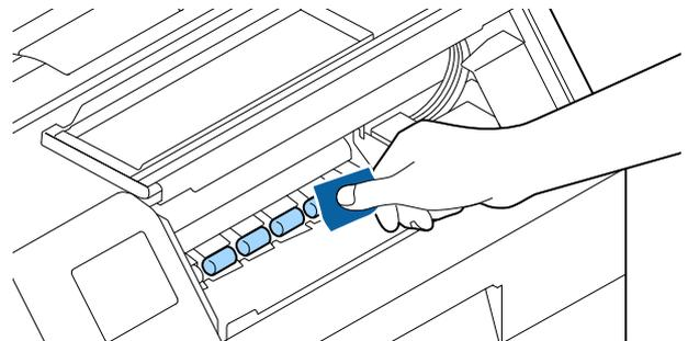
**7 Rotating the roller by hand, remove paper dust or adhesive from entire surface of the roller.**
