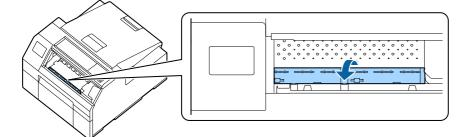
**5** Use a cloth or cotton swab to remove adhesive adhered to the platen.
