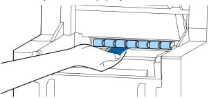
7 Rotating the roller by hand, remove paper dust or adhesive from entire surface of the roller.
