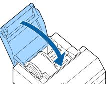
**12** Hold down the Feed button until the leading edge of paper touches the table on which the printer is installed.
