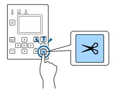
**3** Press the Back Feed button to feed the paper backward.
