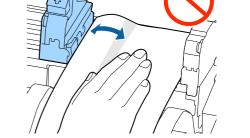
8 Insert the paper into the paper feed slot until paper feeding starts automatically.
