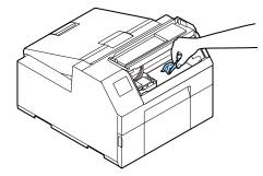
4 If the print head is not on the far right, hold it down and move it to the far right. If there is jammed paper, remove it.
