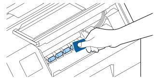
Rotating the roller by hand, remove paper dust 7 or adhesive from entire surface of the roller.
