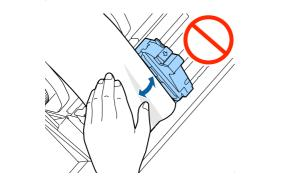
9 Insert the paper into the paper feed slot until paper feeding starts automatically. Do not load backing paper that has no labels on it. The
