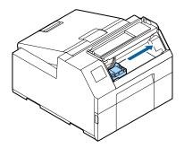
5 Open the paper cover. Raise the release lever. 6 Pull the paper out from the paper feed slot. 7 Lower the release lever. 8 Close the paper cover. g Close the front cover. 10 Press the Pause button. 11 The paper jam error will be cleared. To resume printing, load the paper again. ( Thow to Load Paper (Auto Cutter Model - Supply from Inside)" on page 39, "How to Load Paper (Auto Cutter Model - Supply from Outside)" on page 41)
