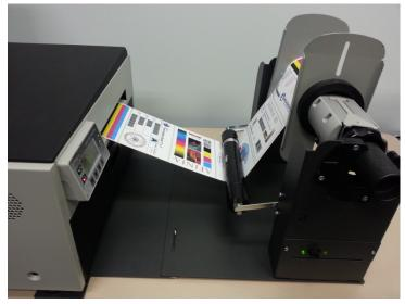
10. Press the Resume button on the printer front panel to resume the print job.
