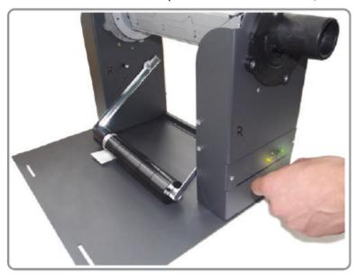
6. Move the tension arm about 2/3 of the way to the top and insert the clip to press the button again. The green LED will be flashing.
