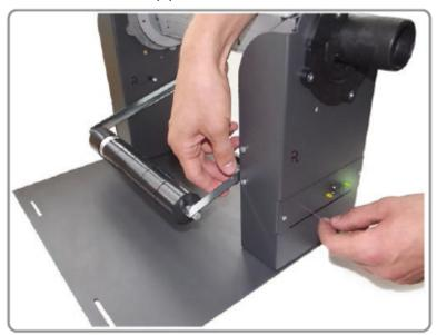
7. Move the tension arm to the highest position and insert the clip to press the button again. The holder will start rotating.
