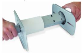
3. Tighten down the core by turning the dial on the motorized core holder counter clockwise.
