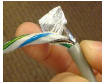
Figure 2: To minimize emissions with the optional PS1 Power Supply module, optionally use a shielded power conductor.
