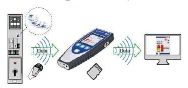
The UltraTEV Plus² has NFC capability to store Asset data on programmable tags. It also has the ability to transfer the results directly on to your PC via Wifi or USB / SD Card. The survey functionality allows details of substations and assets to be entered on the screen, guiding users through the simple survey process. Screen shots can also be captured and saved.
